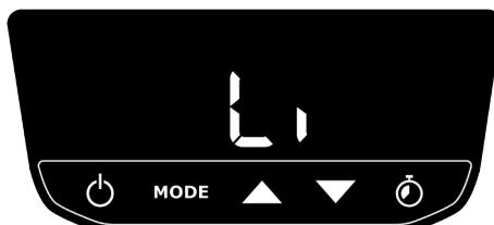
The user must select the measurement scale, either degrees Celsius (°C) or degrees Fahrenheit (°F), in order to complete the configuration. Select the required option using the up or down buttons on the control panel or remote control and confirm with the ON/OFF button on the unit. After this last confirmation, the unit will go off and remain ready to power up.
