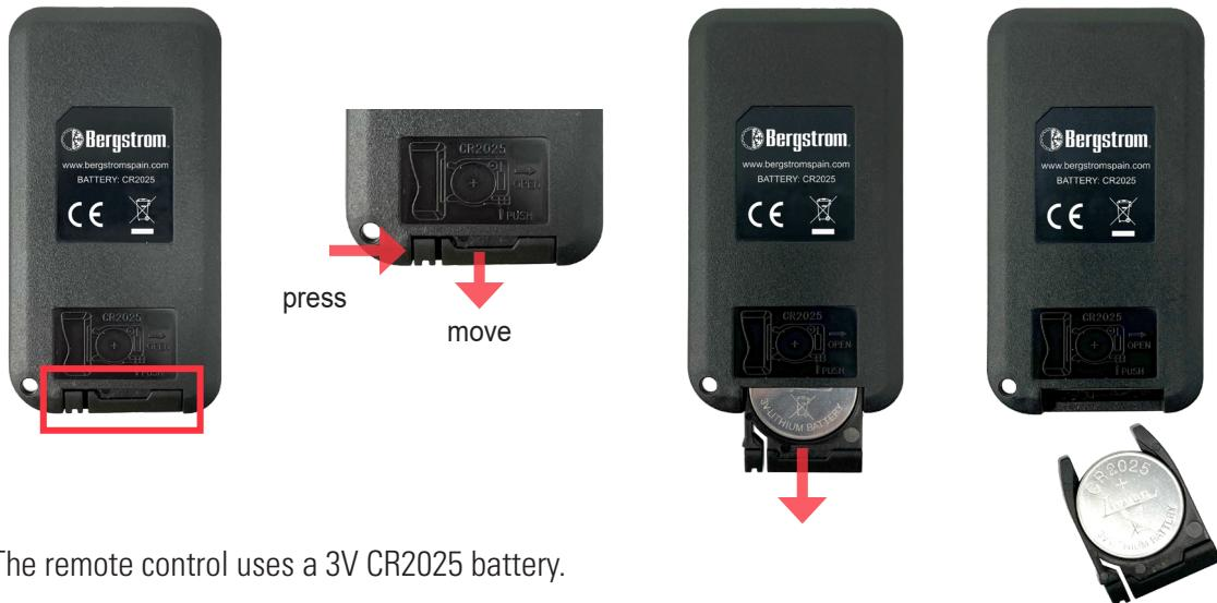
The remote control uses a 3V CR2025 battery.
