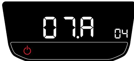
After a few seconds, it will enter initial configuration mode in order to select maximum unit power between 1.2 (1230 W) or 2.0 (2020 W) from the control panel. Select the required option with the up or down buttons on the panel or remote control and confirm by pressing the ON/OFF button on the unit.
